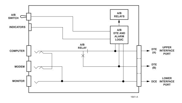
Figure 2-5. LED/Alarm Patch Module with A/B Switching Simplified Circuit Diagram
